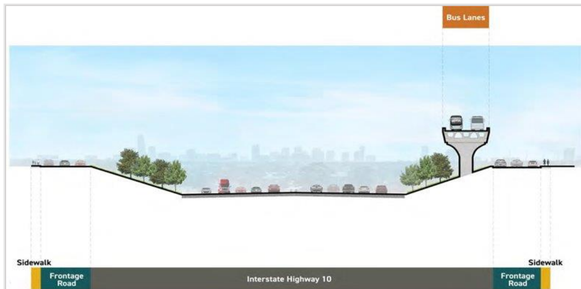
Exhibit 3-2: Typical Cross Section of the Elevated Busway
